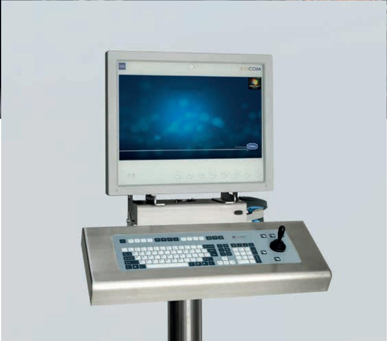
SHARK operator station with barcode scanner and integrated RFID module
