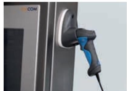
Barcode scanner at monitor enclosure
