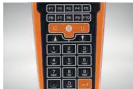
Membrane keypad with 10 function keys
